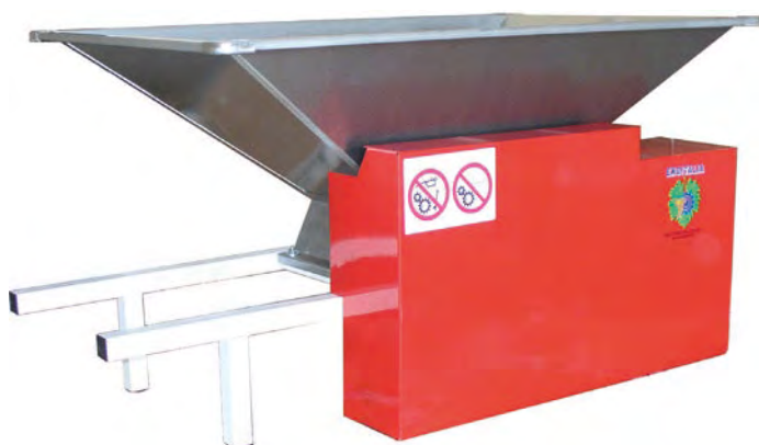
ENO 1, ENO 2 - Stainless steel hopper, with engine
